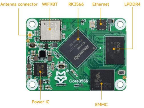
Core3566 highly integrates the function of Rockchip RK3566 quad-core processor in a compact board. RK3566 integrates quad-core A55 CPU, dual-core ARM G52 GPU, VPU, NPU, supports video output, PCIE, CSI and other interfaces, and is very suitable for For embedded applications, different RAM, eMMC flash memory specifications and wireless module specifications are available.
